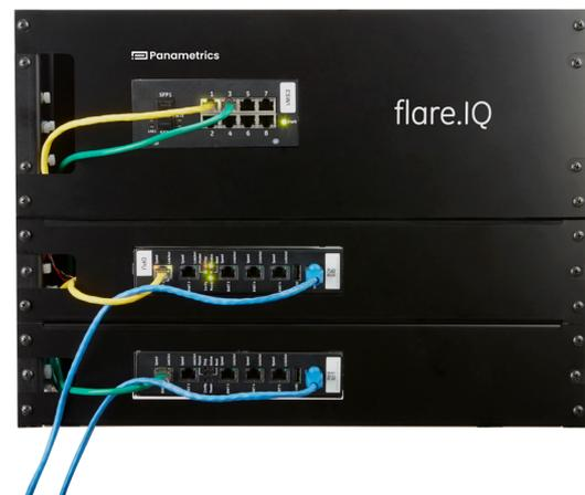
Made by Baker Hughes, Panametrics' flare.IQ offers a plug-and-play answer to companies' needs, from meeting regulatory standards to helping harvest LNG to achieving maximum efficiency from flares. Flare.IQ is housed in a Windows-based industrial controller that seamlessly interfaces with existing distribution control systems.
